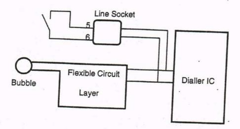
Figure 1. Hookswitch configuration in the TF200
