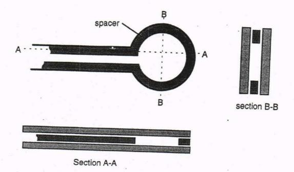
Figure 2. Diagram of hookswitch Bubble construction
